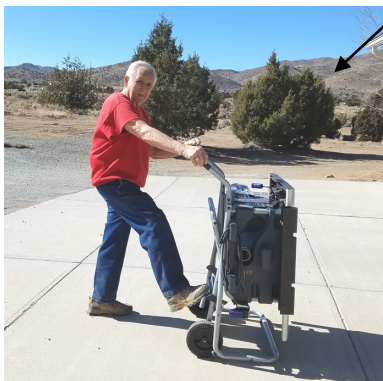
Stepping on the pedal to lower the saw
